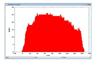
The axes of the plot are the *number of the trajectories* (y) and the id of the periods (x).
